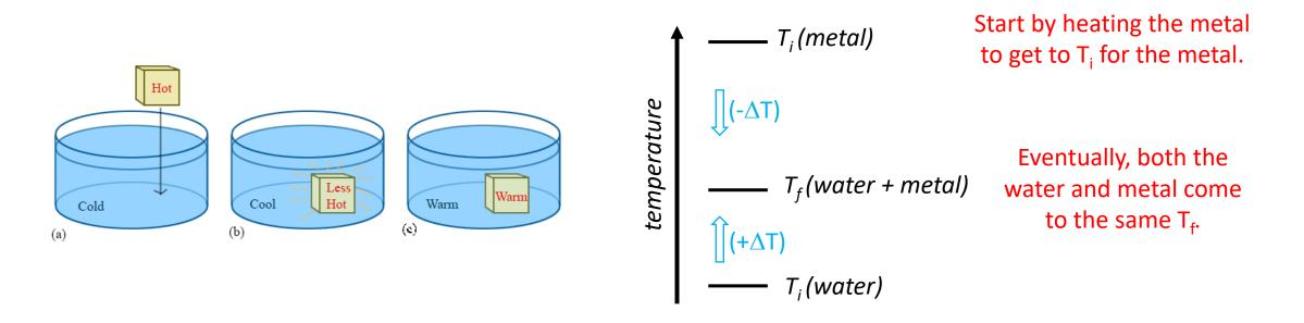
• After they reach the same T<sub>f</sub>, the heat lost by the metal equals the heat gained by the water.
